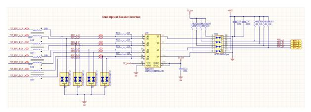
When applied to a 2D scanning system then the digital inputs for a quadrature encoder are assigned as follows:
